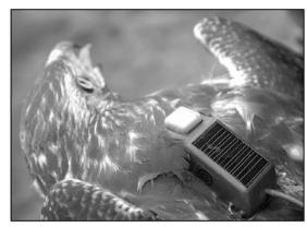
The 20-gram, GSM transmitter lines up in the middle of the bird's back and is held in place with Teflon tape which will wear and fall off eventually. [Photo by Mason Cummings]
